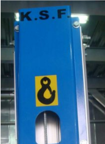
cable under steel crank-case and crane lifting point for safe transportation
