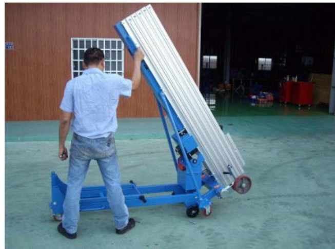
Easy tip of the mast for easy horizontal or vertical transport
